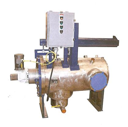
This unit has rails to aide in the removal of the screen and in the adjustment of the scraper blade. When adjusting the scraper blade, the screen can be manually turned for fine adjustment. The screen and scraper blade is a one piece sub-assembly. All screens are fabricated and machined for a tight tolerance and true running surface. The blade can be manufactured from various metals and plastics.
